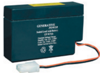
Compact 12 Volt Sealed Lead Acid Battery • Output: 12 VDC / 800mAh
